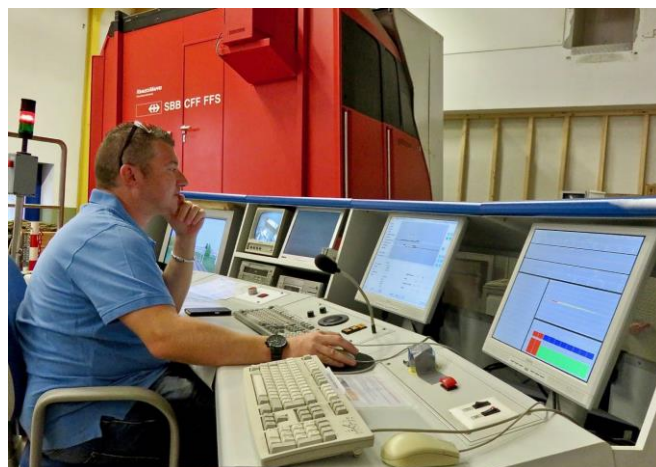
Figure 2: In the DESM laboratory, a complete simulator for human-in-the-loop testing has been developed. The simulator can be configured according to the needs of the experiments. A driving cab of a Swiss locomotive type Re 460 is pictured above. The subjects are situated in an exact replica of their workplace environment, where they can perform as they do in real life work situations
