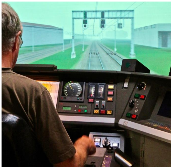
Figure 1: The holistic simulator for train drivers allows for the investigation of human performance under special and extreme conditions, which is not possible in reality. The repetition of such experiments makes it possible to apply statistical methods to allow for the evaluation of the collected data
